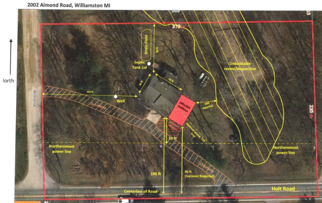
Sketch plan provided by the applicant which shows existing conditions and proposed location of the addition.
